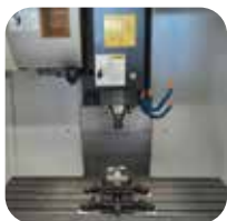
Spindle direct drive 12.000 rpm
